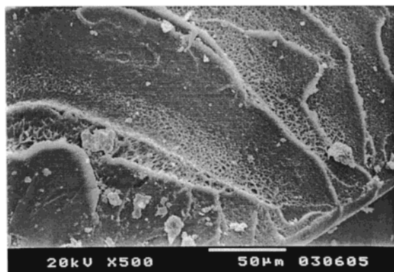
Figure 11. SEM micrograph of the fracture surface of cold drawn PEN along a big shear band.
